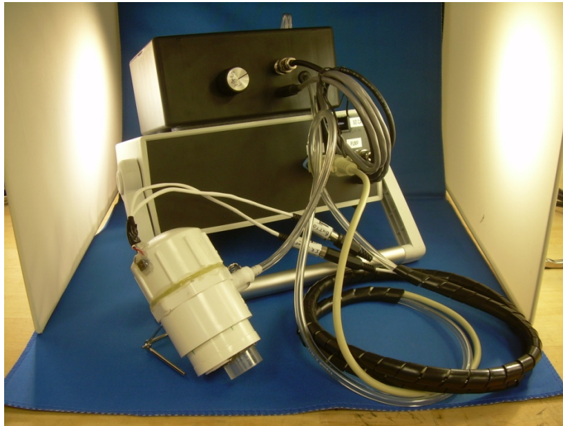
Figure 3.3: A working prototype of the Cutisfirm Skin Tension Measurement System. A Sharp GP2D120 IR proximity sensor is housed in a suction probe made of PVC fittings and a clear acrylic nozzle for skin attachment. The probe is attached to pump/value control electronics boxes.
