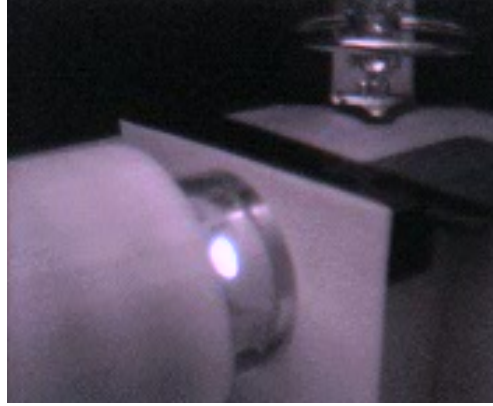
Figure 3.6: Image of IR beam spot from proximity sensor in a Cutisfirm prototype. Using a webcam with the color filter removed, the approximate 850nm beam spot from the IR proximity sensor, with the 1mm-hole attenuating cap installed, is shone on a piece of yellow paper and seen through the clear acrylic tip of the probe.
