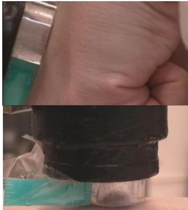
Figure 3.25: Images of skin deformation on the back of the hand in different positions: fist hand (upper) and relaxed or flat hand (lower) taken by a video camera. The green ruler is used as a reference distance in image analysis using Image J (NIH Open Source Image Analysis with JAVA).
