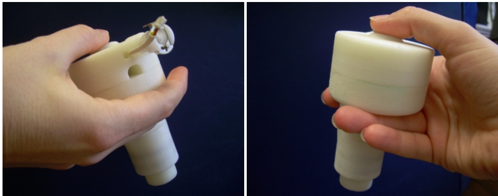
Figure 3.1: Images of the skin testing probe proposed design. Housed inside the probe is the Sharp GP2D120 IR proximity sensor which will produce an IR beam that will be reflected off of the skin and then received by its CCD linear array IR detector to determine skin deformation.
